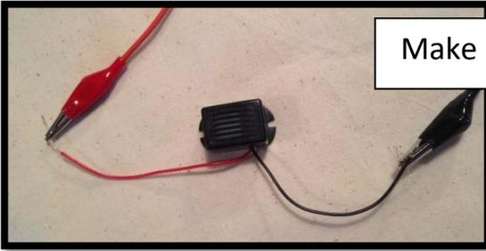
Make a simple circuit with a buzzer.
