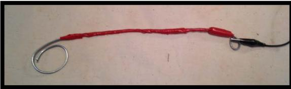
Make a hook using wire. Wind electrical tape around to create a handle. Twist the wire at the ends to stop the sharp point from sticking out. Make the loop at one end larger. Make a break in the circuit and add the hook in.
